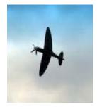
the spitfire, with its elliptical wings, focuses lift as far as possible from the tip of the wing to prevent leakage.
