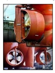
In this case the shroud can provide up to 50% higher yield. Because the loss tip blades are no longer feared the chord blade tip can be great, because the blade keeps its effectiveness through the tip. The shroud generates a drag proportional to the square of the speed of the ship. Above a certain speed of evolution, gain efficiency losses in the end of the blades, will be destroyed by the drag generated by the shroud. The shrouded propeller is therefore suitable for low speed vehicle.
