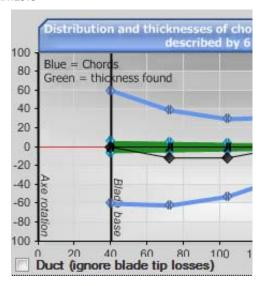
This is not completely realistic because the friction between the blade tip and the fluid stationary in the boundary layer of the shroud, will be added and affect the torque so the performance will be affected. In practice we keep a gap greater than the boundary layer of the shroud, implying that leaks can persist....So HELICIEL gives you in this case, performance slightly overvalued. But it is still usefull to asses the benefit of a shroud around the propeller
